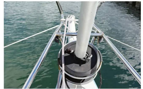
The original pulpit was smashed and had to be rebuilt. A bowsprit was added to accommodate an asymmetric spinnaker and a Profurl furler
