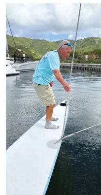
The stainless steel standing rigging has been replaced with Colligo Dux brand Dyneema for the shrouds and regular Dyneema for the rest. Antal low friction rings with Dyneema lashing lines make tension adjustments easier around the new chainplates
