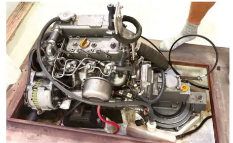
A Yanmar 30hp diesel engine fitted post-Irma ensured Triple Jack was compliant with race rules for the 2024 edition of the Caribbean 600
